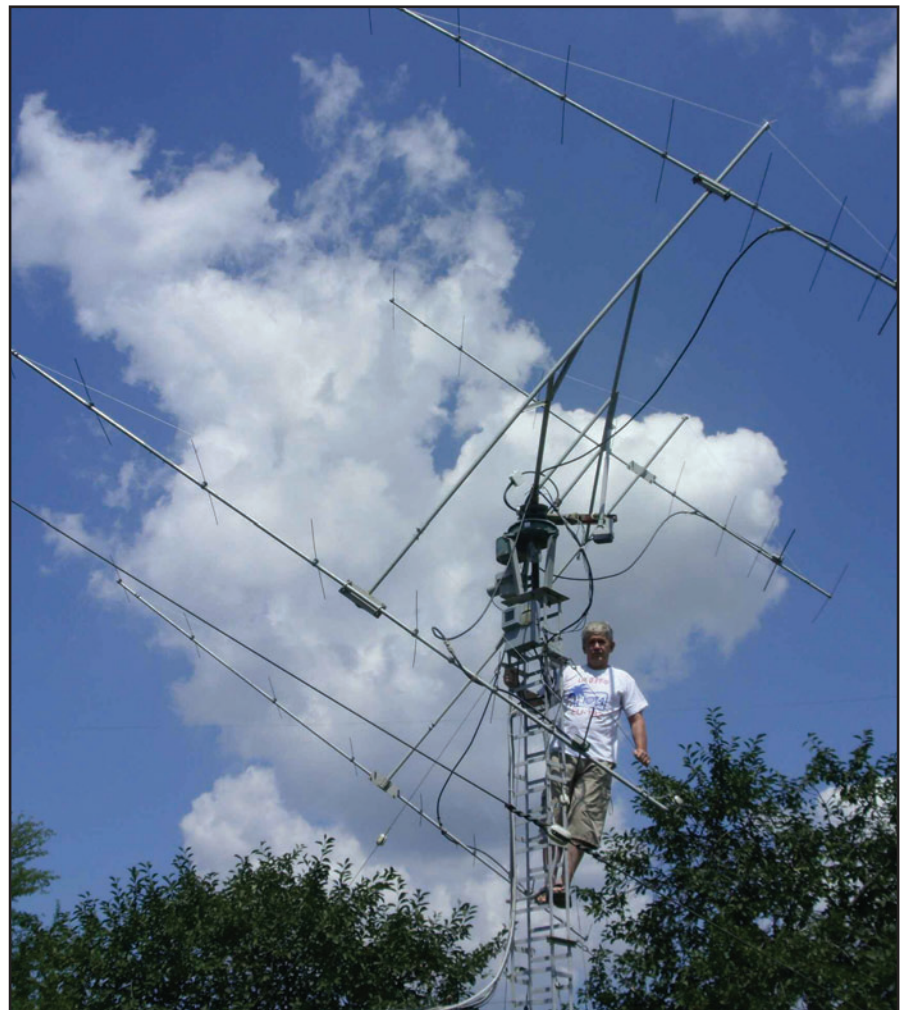
UXØFF's 9-element array helped him to the DX #1 spot on 2 meters.
