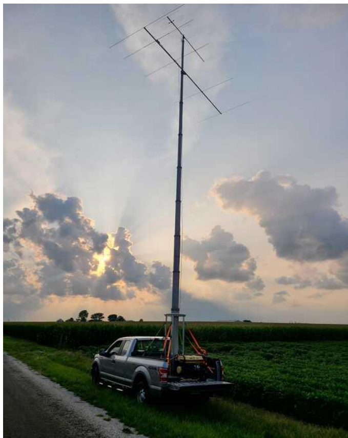
AC0RA's outstanding rover setup built around a pneumatic mast holding large 6 and 2 meter Yagis
